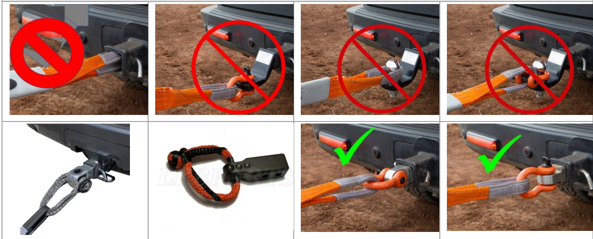
Figure 2 – Rear anchor points – Light duty vehicle with a hitch and soft or hard clevis. Hard clevis usage must be approved by Supervisor
