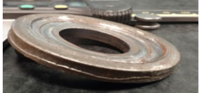
Figure 15 - Eye bolt flat washer cupped due to overtorque
