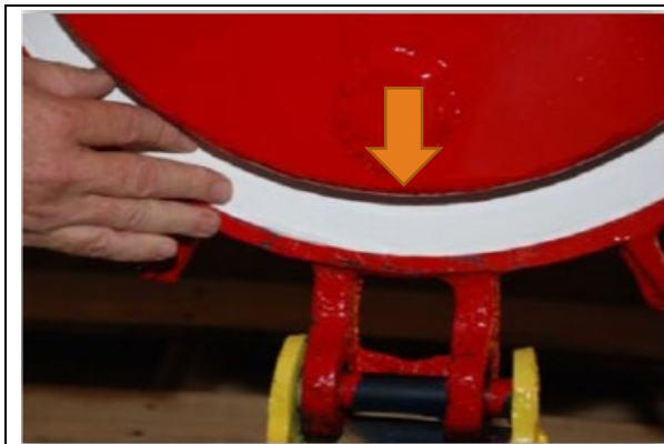
Figure 9 - Manway Cover Gasket
