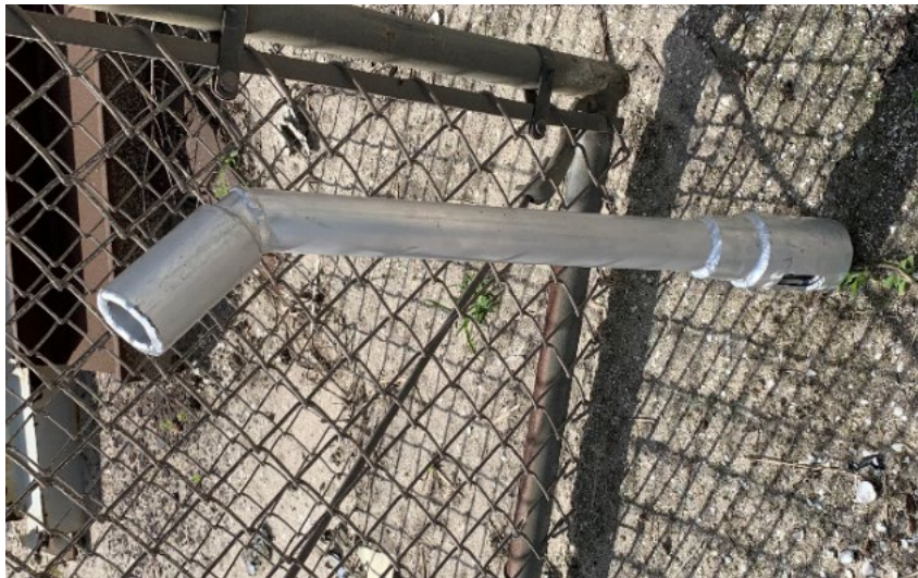
Figure 2 - Valve Handle extension - Aluminum
