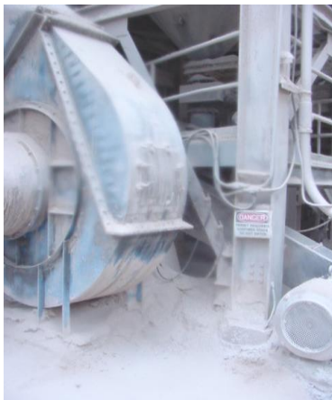
Large Blower – Only a confined space if the rotating element is removed.
