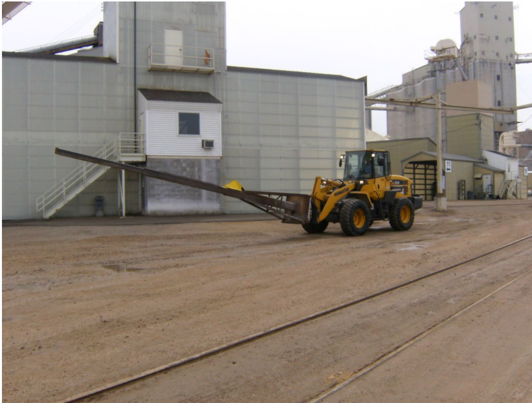
Figure 1 - Typical probe attached to a payloader.
