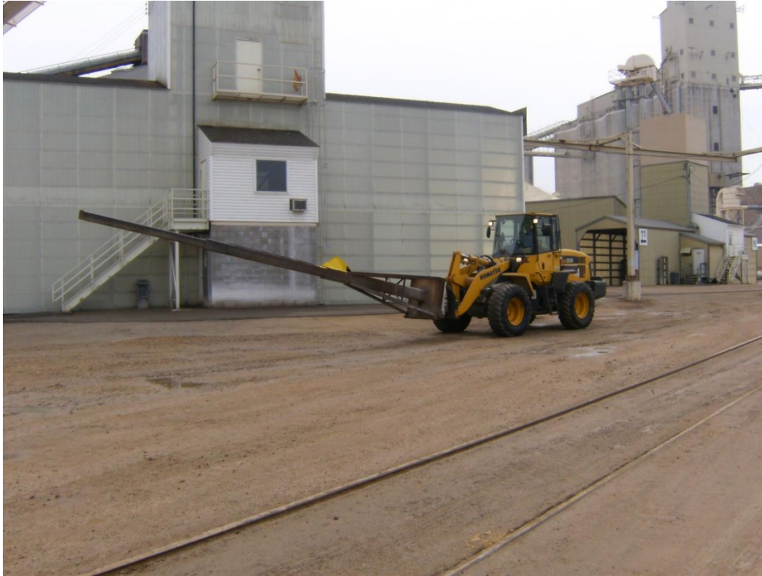
Figure 1 - Typical probe attached to a payloader.
