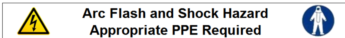
Figure H- 10 - Pictorial Panel of a Mosaic Detailed Arc-Flash Label
