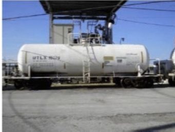
Figure 1 - Sulfuric Acid Railcar Loadout
