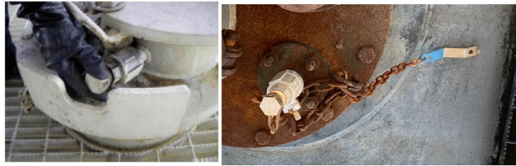
Figure 32 - Remove handle from air valve if car dome doesn't have a protective housing
