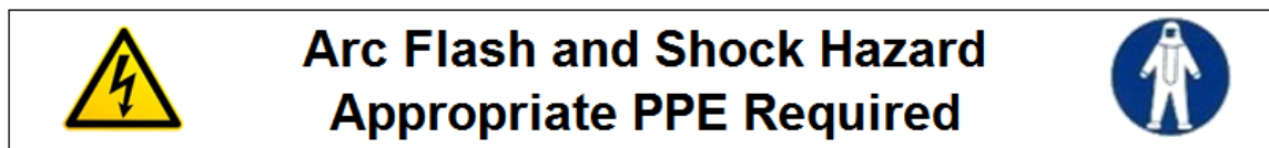
Figure H- 10 - Pictorial Panel of a Mosaic Detailed Arc-Flash Label
