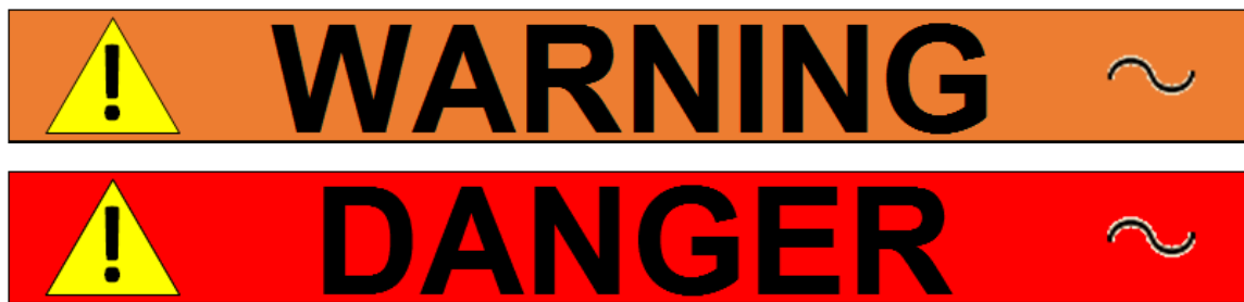
Figure H- 9 - Header Panel of a Mosaic Detailed Arc-Flash Label
